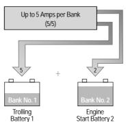
Competitive chargers have an amp limitation per bank. As illustrated the (5/5) 10 amp charger can not transfer the unused 3 amps not required by the engine start battery, leaving only a maximum of 5 amps for the trolling motor battery.
