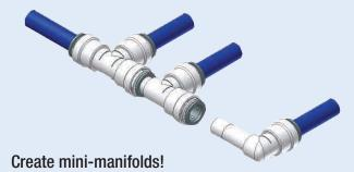
With AquaLock fittings, small lengths of tubing can be eliminated by using our stackable connector configurations. Simply snap together Tees and/or Elbows to create a mini-manifold of fittings. Because AquaLock connectors rotate, the direction of the tubing can be oriented by a simple twist, reducing the amount of tubing required to plumb a water system.
