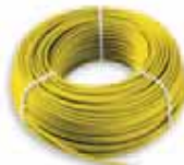
01840.Y Bus buglar alarm system cable, halogen-free 2x0,50 mm 2 , rated operating voltage to earth 400 V, suitable for I category cables, yellow - 100 m
