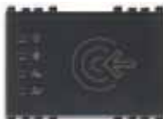
19457 Transponder card reader for installation outside rooms, KNX standard, 2 NO 4 A 24 V- relay outputs, 2 inputs, power supply 12-24 V~ 50-60 Hz and 12-24 V d.c. (SELV) - 3 modules. Supplied without transponder card
