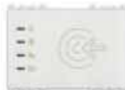
19457.B Transponder card reader for installation outside rooms, KNX standard, 2 NO 4 A 24 V- relay outputs, 2 inputs, power supply 12-24 V~ 50-60 Hz and 12-24 V d.c. (SELV) - 3 modules. Supplied without transponder card
