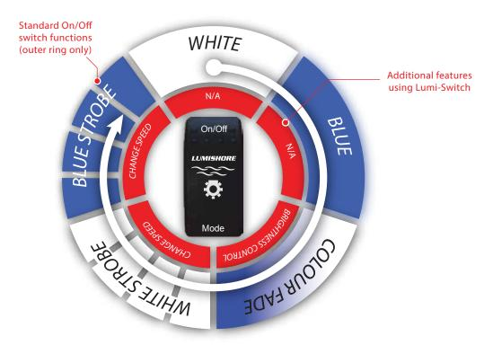
Note: The SMX SUPRA lights have built in memory. When they are switched on for more than 30 seconds, the setting will be saved. The lights will have the same setting next time they are switched On.
