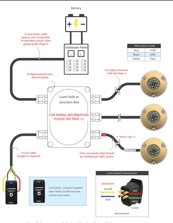
Note: Only one master light should be installed per light system
