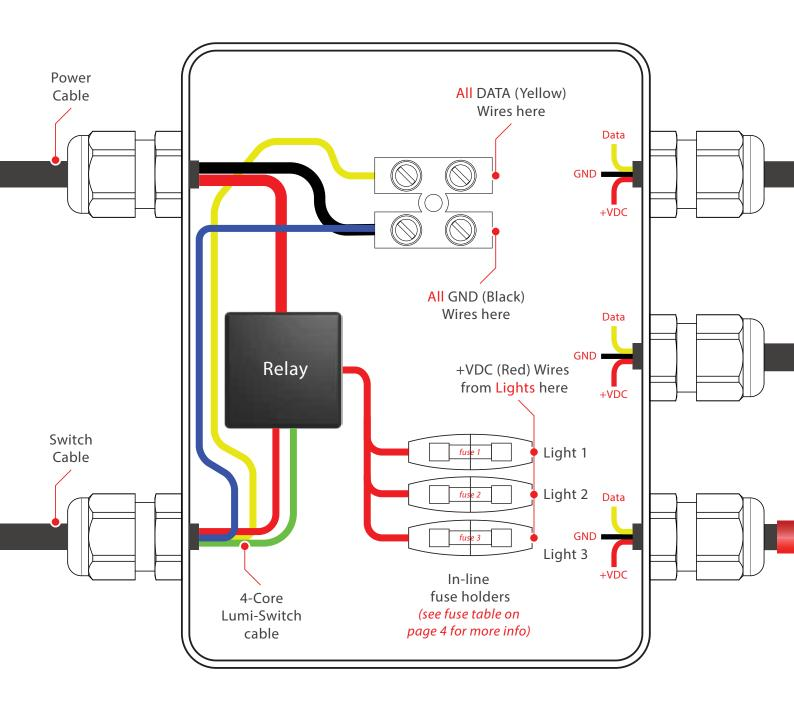
Note: For a system with more than 2 lights, or for cable runs over 4m. A marine grade Relay should be installed. Check the voltage rating is suitable for your Vessel (12/24V). The power requirement will depend on model and number of lights installed per relay. Consult table on page 4 for Amp rating of each light
