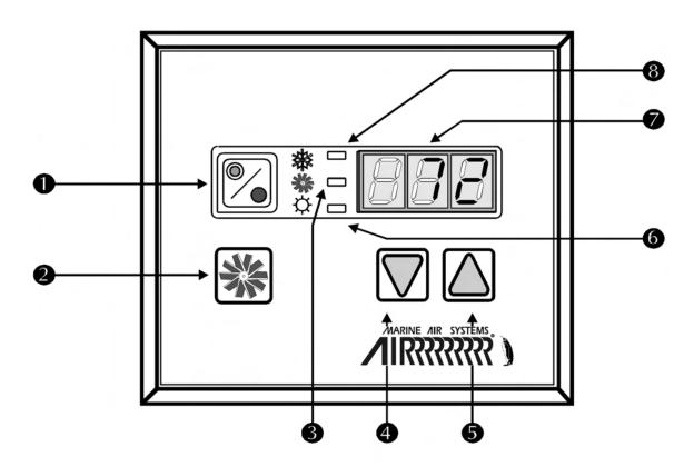
**Power & Down Buttons...** Simultaneously press the Power and Down Buttons while in the On Mode to enter the Moisture Mode.
