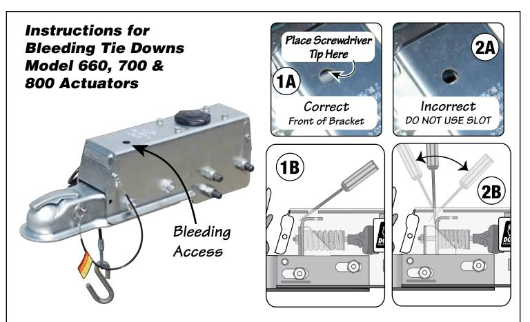
To pump master cylinder, insert a flat tip screwdriver into the round hole near the front of the actuator cover (See 1A). The screwdriver should be at the lowest angle possible to the actuator so that it slides in front of the e-stop bracket (See 1B). Screwdriver tip MUST BE IN FRONT of the e-stop bracket and NOT in the slot on the e-stop bracket (See 2A). Push the screwdriver forward and back to pump the master cylinder. (See 2B).
