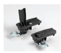
The composite Lift & Turn latch is a light- to medium-duty latch, utilizing engineering plastic in its major components to reduce weight yet maintain excellent strength. When the lever is in the upright position, it rotates 360° to move the cam behind the support in any one of three 90° positions. Once in place, the lever closes flush with the housing, providing 5 mm of axial pull, locking the device with an over-center action.
