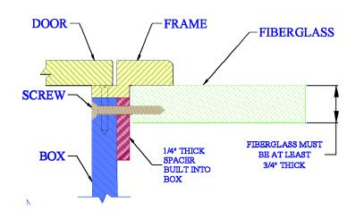
Please Note: Inside Mounting allows you to mount your box without any visible fasteners; however it can be a slightly more involved installation. If preferred, any box that comes predrilled for inside mounting can easily be mounted using face mounting by simply drilling and countersinking your own mounting holes through the face of the frame. View Face Mounting Instructions
