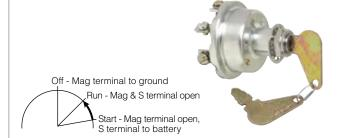
Key removable in Off position, spring return to RUN. Self-grounding in the Off position in metal panels.
