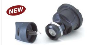
Tested to SAE J259 for ignition switches. Plastic facenut and nickel-plated brass backing nut. Supplied with two matching double bitted keys, with or without TPE (thermoplastic elastomer) key boot. Mounting stem M22 x 1.5 is 0.85" long (21.6mm) and 0.87" diameter (22.0mm ). Double-D mounting hole is 22.5mm diameter with two flat sides at 9.75mm from the center, Maximum panel thickness 8mm, For replacement keys see page 5. 10A at 12V DC, 5A at 24V DC.
