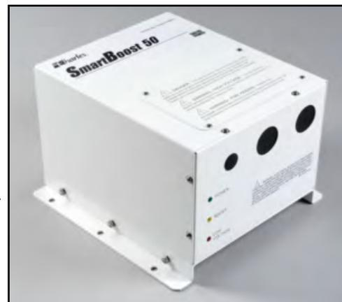
The SmartBoost is a universal AC voltage booster designed to increase incoming AC shore power voltage. When dockside power drops below 208 VAC, SmartBoost provides a 13% AC voltage boost to any existing 50 Amp transformer. Designed as a separate boost control unit, SmartBoost may be connected to any manufacturer's 12 kVA or 15 kVA (50 Amp) isolation transformer.
