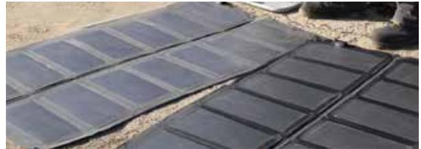
Solar power option panels fold for stowage on top of the backpack frame
