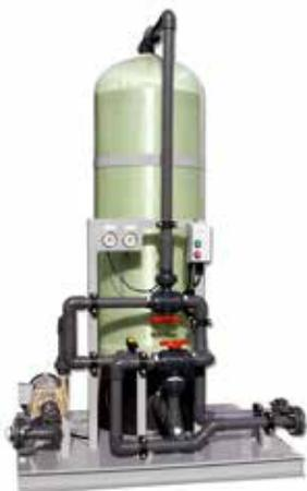
Parker Village Marine Media Filtration Systems offer multi-media performance and are specifically engineered to operate with Village Marine PW Series Watermakers. The media layers are optimized to remove particulate matter from the feed stream ahead of the micron filtration system.
