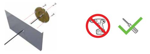
IMPORTANT: DO NOT OVER TIGHTEN. DO NOT USE POWER TOOLS TO TIGHTEN SCREWS.
