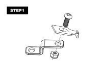
1. Install "Z" shaped bracket threaded on to the Bluetooth controller hook. (packed with Bluetooth controller.)
